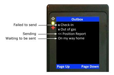
For each message queued in the Outbox, the nano attempts up to three times to transmit. After three failures, the message will be dequeued to avoid draining the battery. User has to <u>manually</u> requeue a message. If the nano is at a location not suited for transmission, user has to monitor the Outbox and repeatedly requeue until the message is successfully transmitted. The  $\triangle$  symbol appears on top of the home screen when there is a queued or dequeued message(s) in the Outbox.
