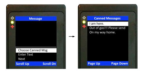
The nano can store up to 600 canned messages. Figure on the previous page displays examples of a few canned messages entered using SatTerm. Each message is shown on a single line. Some canned messages are too long and can only be partially displayed on the LCD screen. User can navigate by pressing the up and down arrow buttons and by pressing the enter button to show the entire message on the Details screen.
