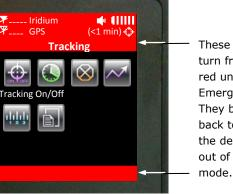
These two bars turn from blue to red under Emergency mode. They both turn back to blue when the device is taken out of Emergency mode.
