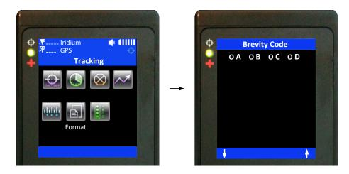
2. When the PECOS format is selected using the Tracking/Format menu, the default Brevity Code setting appears at the bottom of the home screen replacing Check-In and Way Point. The ↓ and ↑ soft keys can be pressed repeatedly to browse through the list of Brevity Codes. The code appeared on the screen will be automatically used by the nano to include in the tracking reports. No further action is needed to select the brevity code.
